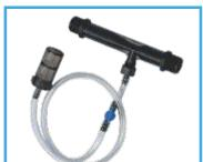
3. 2" Ventury :- It works at 0.5 kg/cm2 differential pressure & capacity of 500 ltr/hr. It also comes with suction tubing, valve & strainer.
