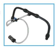
2. 1" Ventury :- It works at 0.4-0.5 kg/cm2 differential pressure & capacity of 50-150 ltr/hr. It also comes with suction tubing, valve & strainer.
